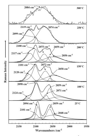
Fig. 6. Hot stage Raman spectra of the 1950 to  $2150 \text{ cm}^{-1}$  region of the hexacyanoferrate(II) interlayered Mg, Al hydrotalcite.
