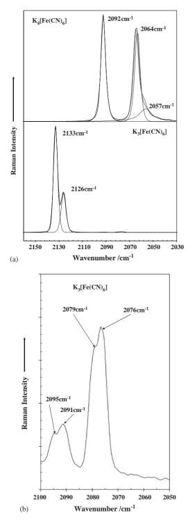
Fig. 2. (a) Raman spectra of the potassium salts of hexacyanoferrate(II) and (III). (b) Raman spectra of hexacyanoferrate (III) expanded in the 2050 to  $2100 \text{ cm}^{-1}$  region.
