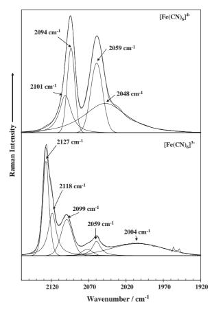
Fig. 4. Raman spectra of the hexacyanoferrate(II) and (III) interlayered Mg, Al hydrotalcite.
