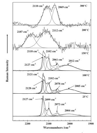
Fig. 7. Hot stage Raman spectra of the 1950 to  $2150 \text{ cm}^{-1}$  region of the hexacyanoferrate(III) interlayered Mg, Al hydrotalcite.
