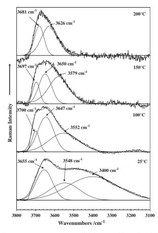
Fig. 5. Hot stage Raman spectra of the OH stretching region of the hexacyanoferrate(II) interlayered Mg, Al hydrotalcite.
