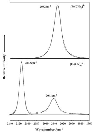
Fig. 3. Infrared spectra of the potassium salts of hexacyanoferrate(II) and (III).
